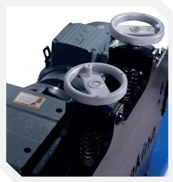
The Rope Drive Machine Type-2 is specialized equipment developed to quickly and efficiently place steel ropes into the formwork before concrete pouring in the production of prefabricated bridge girders. It has the capacity to lay steel ropes with diameters of 0.5 and 0.6 inches and provides speed control in the 0-50 Hz range thanks to its inverter conversion system.
