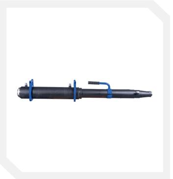
The Tensioning Jack is a YGM-K25 Stork model with a capacity of 25 tons, featuring a stroke length of 400 mm and a 3-effect structure. While performing tensioning and loosening operations in the first two stages, it reduces preload loss by pushing the core inside the cylinder when the pulling is completed in the third stage.
