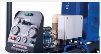
The Hydraulic Multi-Unit is designed as a powerful hydraulic power unit, featuring a machine where pressure settings can be independently displayed on separate pressure gauges. This feature provides the operator with detailed control over the system. Additionally, its ability to use dual jacks offers flexibility for various applications.
