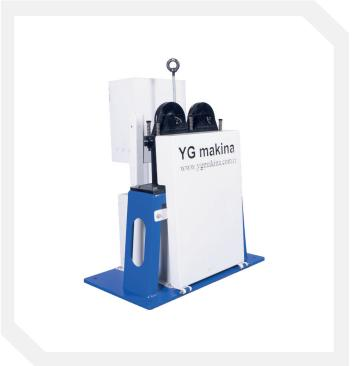
The Rope Drive Type - 1 machine is a specialized piece of equipment used in the manufacture of prefabricated bridge girders, designed to quickly and efficiently place steel cables into the formwork before concrete is poured. This machine has the capability to pull 0.5-inch and 0.6-inch steel cables. Operated by a single person, this machine eliminates manual labor and time loss, making the process more efficient.
